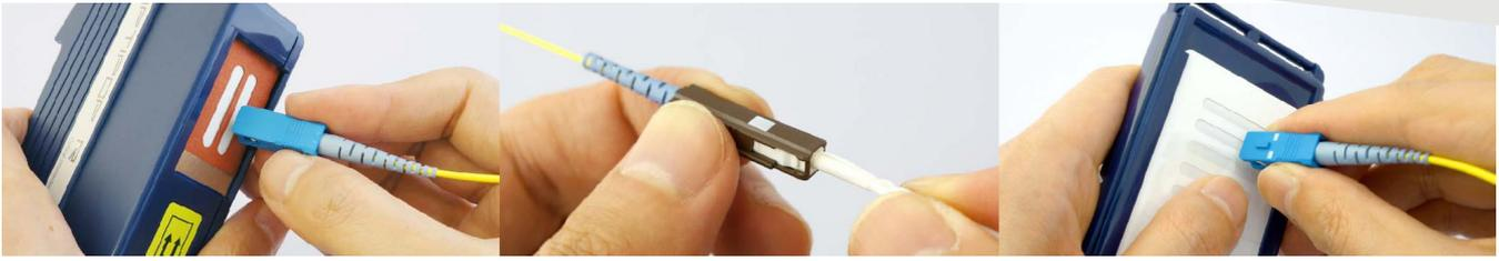
**POINT1** Removes dirt you can't even see without scratching the end face Because they use pure sterile microfibers, they remove dirt without scratching the ultra-fine core of the optical fiber.
